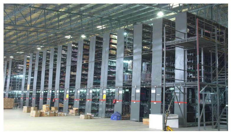
Multi-Tier shelving and racking is mainly used for storage and order picking of non-palletized goods. It is also widely used for other storage units containing small parts/components, bins, cartons and for bulk storage. The modular system accepts numerous accessories which can also be added later on. Designed to suit diverse requirements, these accessories allow storing of almost all goods.
